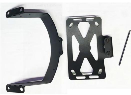
Using the two 1/4"-20 screws, assemble the mounting bracket and hardware in the orientation shown below. The tail tidy is now ready attach to the bike's subframe.
